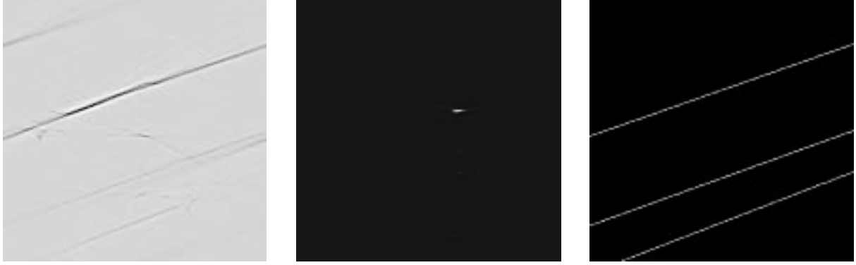
Fig. 12a: Inverse Radon transform of Fig. 10c
