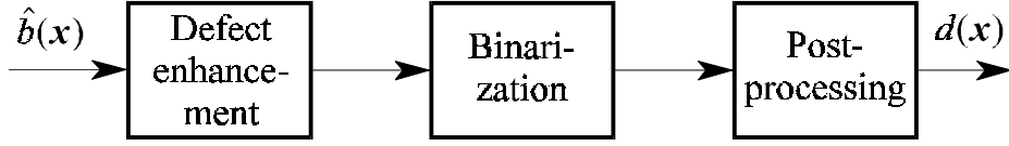
Figure 5: General structure of the local detection algorithms
